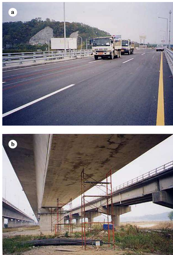
Fig. 8. Experimental work for determination of the dynamic response of PSC box bridge subjected to moving vehicles: (a) dynamic test for moving loads; (b) measurement of dynamic deflections.
